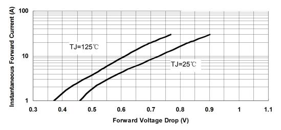
Fig.3-Typical Instantaneous Forward Voltage Characteristics
